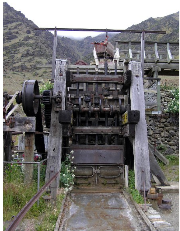
Gravel washed out from the bottom of the machine and the flakes of gold were trapped in the metal pan
