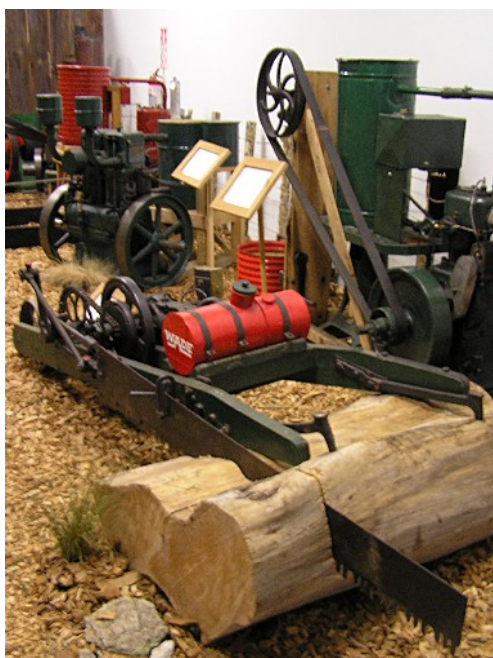
An early petrol driven saw. It was used for processing tree trunks felled by axes
