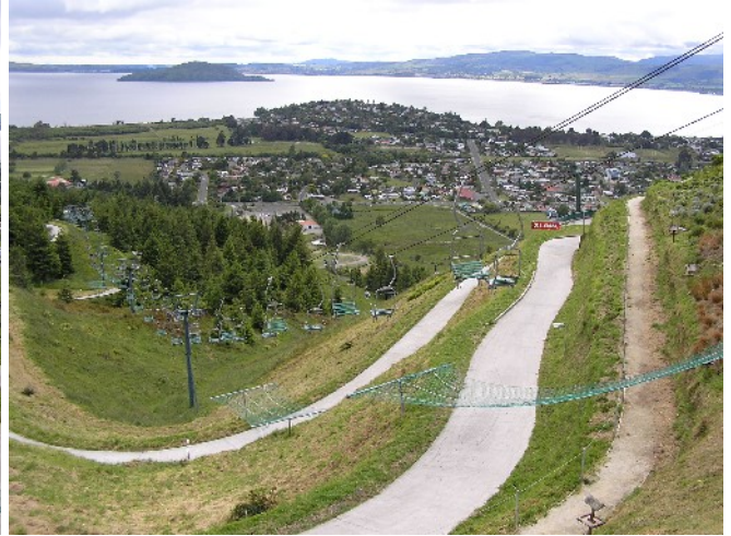
The nets catch things dropped from the chair lift and stop them from falling onto the track
