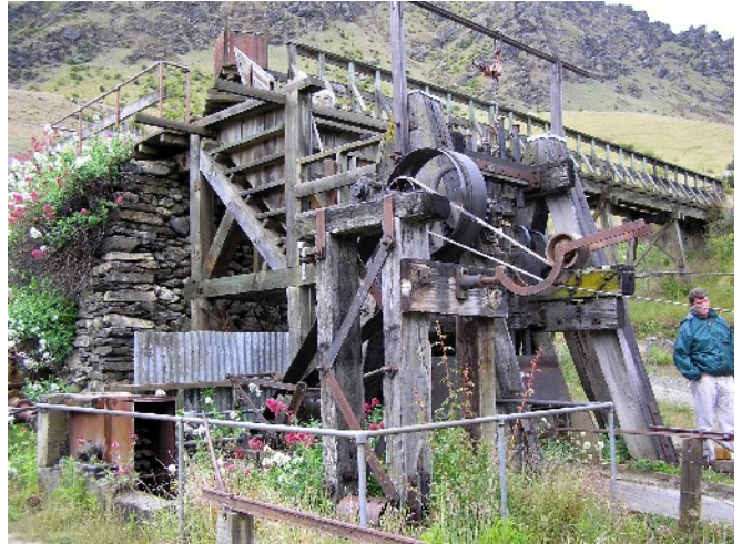
Gold bearing rock was fed into the crusher from the upper trolleyway
